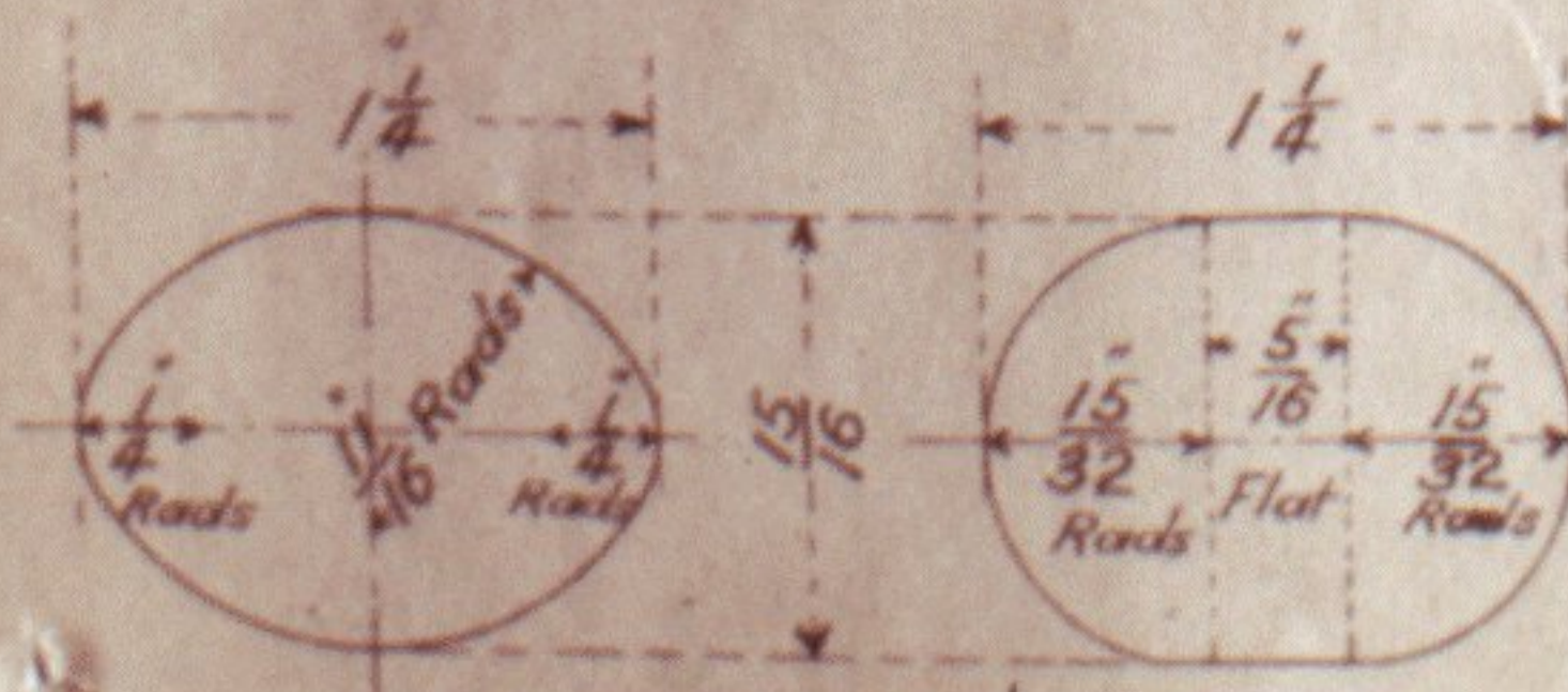
BOLT HOLES THROUGH RAILS.
